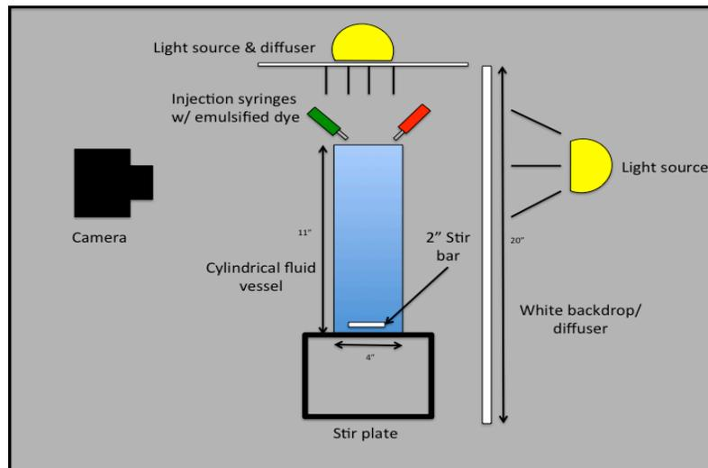
**Figure 1: The complete experimental setup for the stir plate vortex**
