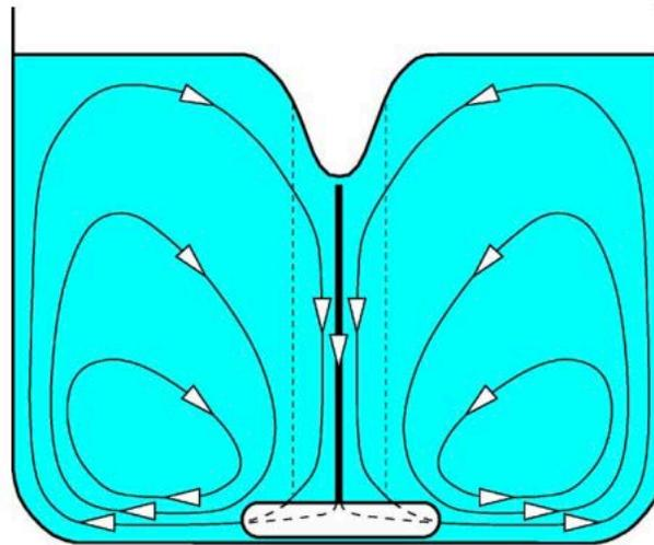
**Figure 2: The resulting convection like current do to the wall bounded flow [3].**
